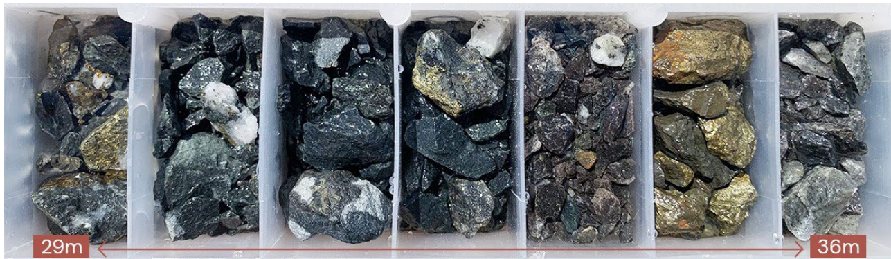
Figure 5. WNR0017; 7.0m (5.6m*) @ 3.58% Cu and 3.96 g/t Au from 29.0m including 2.0m (1.6m*) @ 10.23% Cu and 13.62g/t Au from 34.0m – Wallace North AGC drilling 2023. 6
