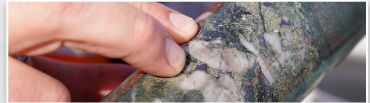
Quartz vein (15cm) with bornite (blue), pyrite and minor chalcopyrite at 221.2m
