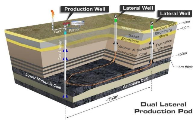
The above schematic provides a visual representation of how Tlou's production pods have been drilled. This is indicative only and not to scale.
