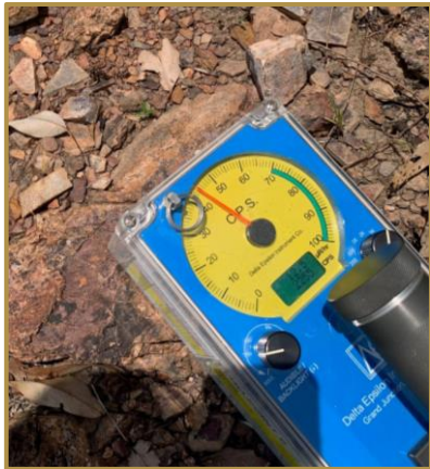
Elevated radioactivity in ferruginous zone measured using scintillometer by Orpheus
