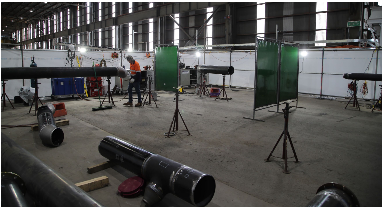
Figure: GEM Industrial pipe workshop on-site for welding of PVDF & CS piping
