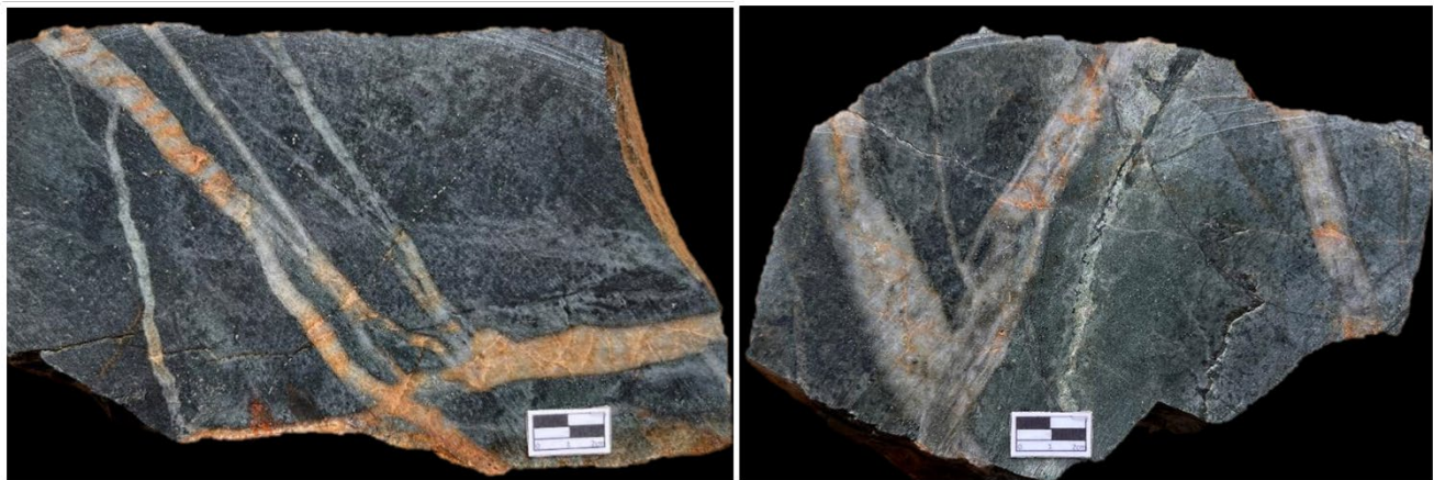
Figure 2: Photos of selected grab samples collected by the Company from outcrop in the area of defined high-magnetic target 3. Left: Sample G1000717 of propylitic altered diorite intrusive with quartz stockwork veins and thin magnetite stringers. Sample contains disseminated pyrite (3-5%) and minor chalcopyrite. Sample assayed 0.44g/t Au, 581ppm Cu. Right: Sample G1000720 of propylitic and silicified diorite intrusive with quartz-magnetite stockwork veins and containing disseminated pyrite (3-5%) and minor chalcopyrite (<1%). Sample assayed 0.47g/t Au, 1,049ppm Cu. See Table 1 for sample location and assay details.
