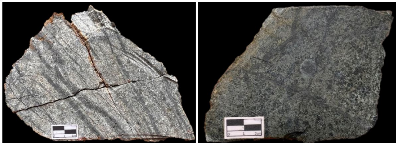
Figure 4: Photos of selected grab samples collected by the Company from outcrop in the area of a defined high-magnetic target at the Jerambah prospect. Left: sample GI000721 of phyllic altered diorite intrusive with quartz stockwork veins and abundant disseminated pyrite (10-20%). Sample assayed 0.06g/t Au, 738ppm Cu. Right: sample GI000722 of propylitic diorite intrusive with quartz-magnetite stockwork veins and disseminated pyrite (3-5%) and minor chalcopyrite and bornite (<1%). Sample assayed 0.08g/t Au, 318ppm Cu. See Table 1 for sample location and assay details.
