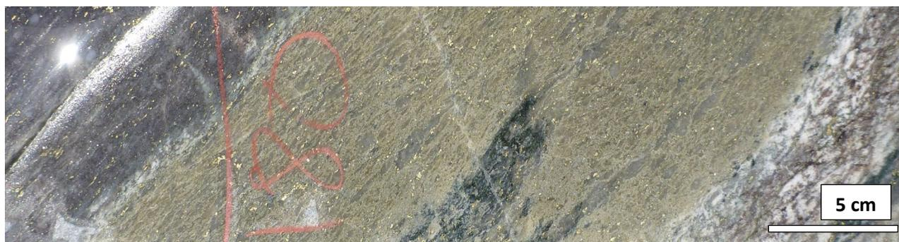
**Figure 8.** Core from CCDD004 (180 m) showing a 20 cm wide zone of intense greenish yellow sericite-chlorite alteration replacing pale brown potassic alteration (left contact) and greyish white albite and forest green actinolite sodic-calcic alteration (right contact). Note the disseminated brassy yellow pyrite and chalcopyrite in the foliations in diorite.
