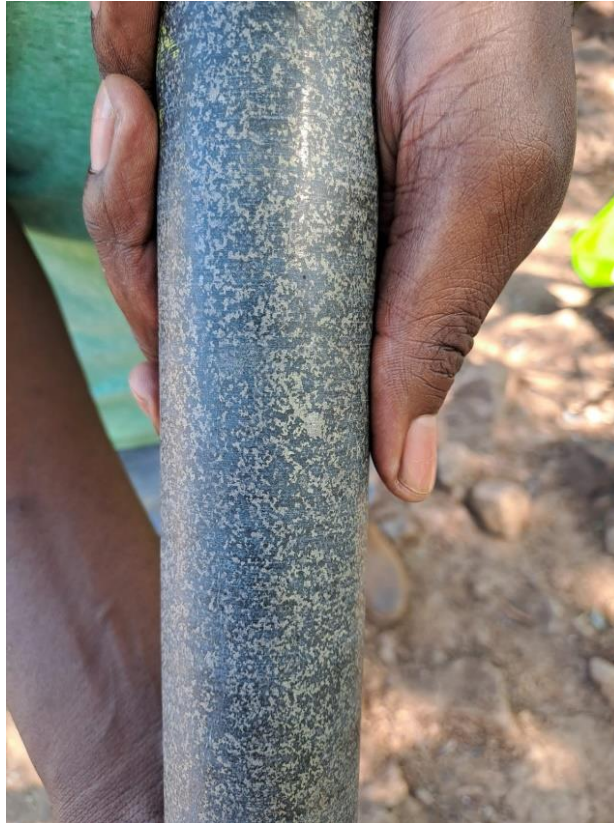
Figure 1: BNDDD002 – 379.38m – accumulate komatiitic dunite with net-textured magmatic sulphides from within a zone where the sample returned 10.33% Ni, 2.24% Cu and 0.10% Co over 0.76m (refer to Tables 1 and 2).
