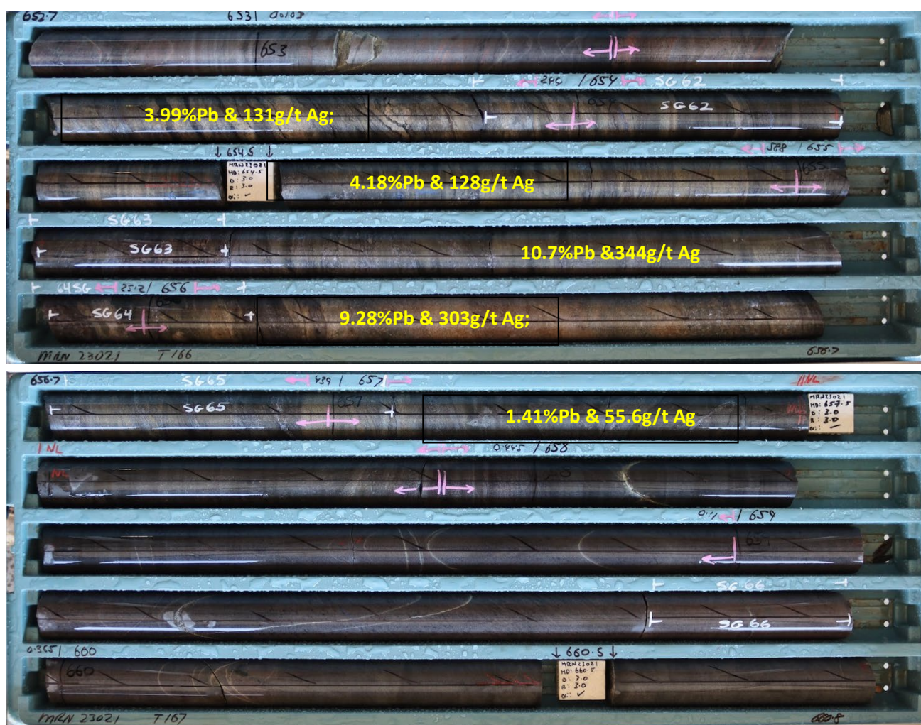
Figure 1:MRN23021 – Drill core shown with lead and silver grades of respective sample intervals from 653.35m – 657.90m assayed 6.2% Pb 202g/t Ag (369g/t silver equivalent)
