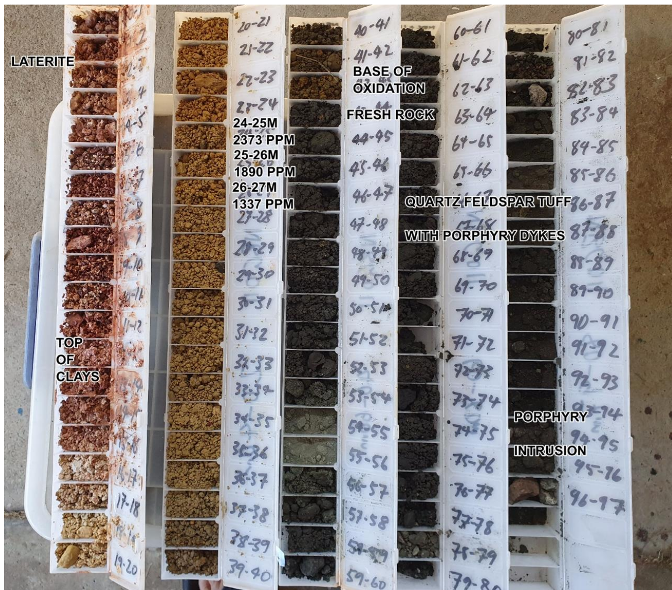
Figure 5: Chip tray photo NBG011 with rare earth oxide intersection
