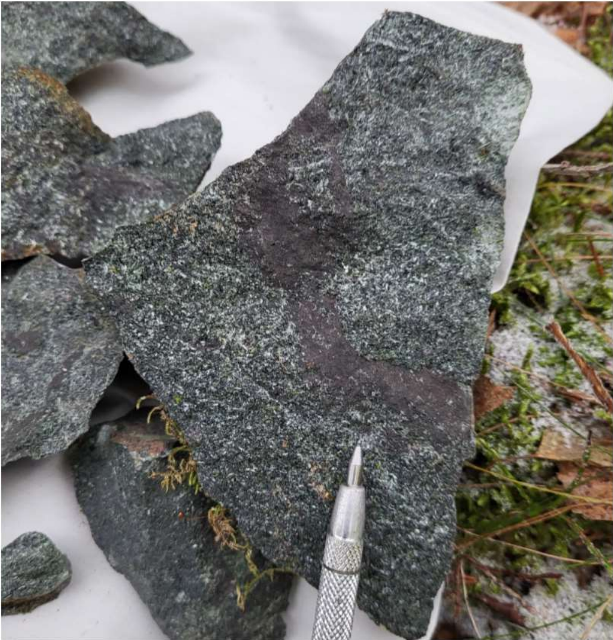
Figure 5: Dark REE vein in green actinolite-tremolite skarn in the project area.
