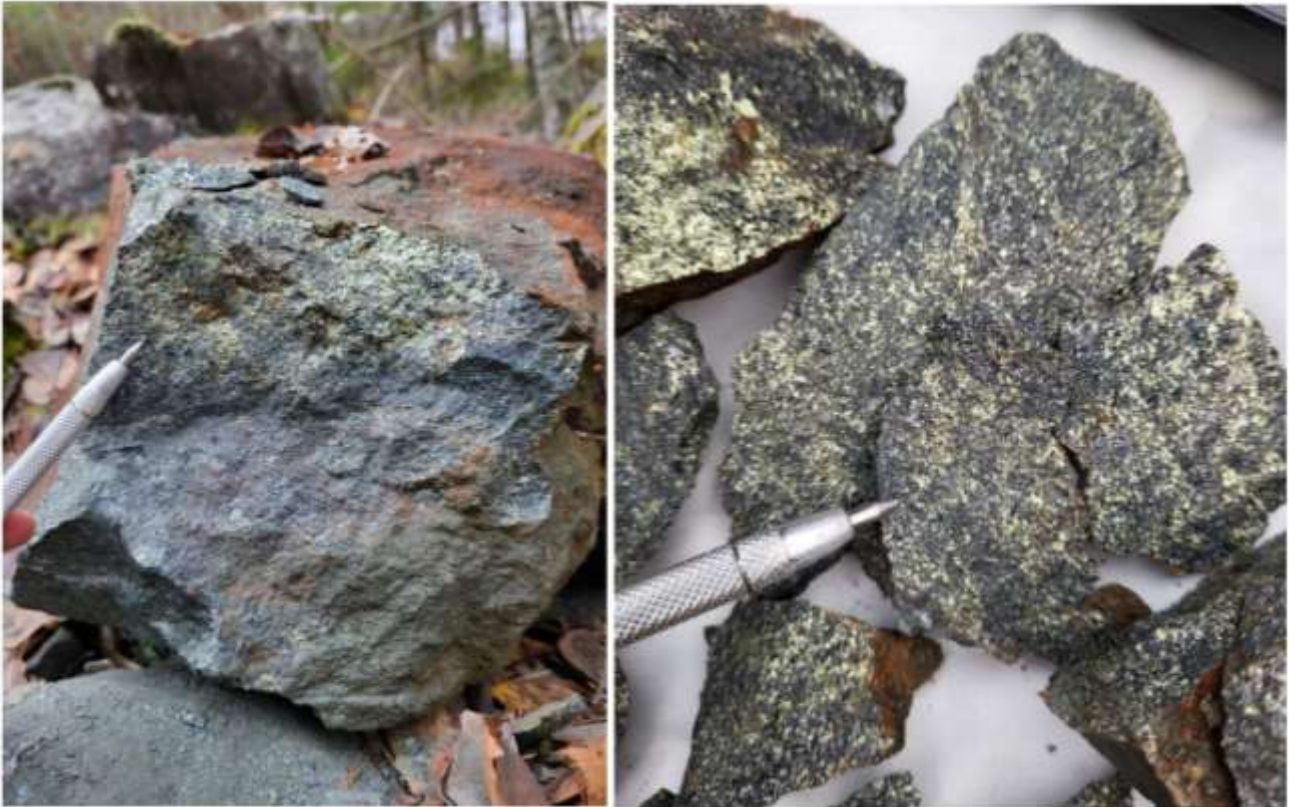
Figure 6: Lenses and clusters of chalcopyrite in massive magnetite boulders (GYTR015).
