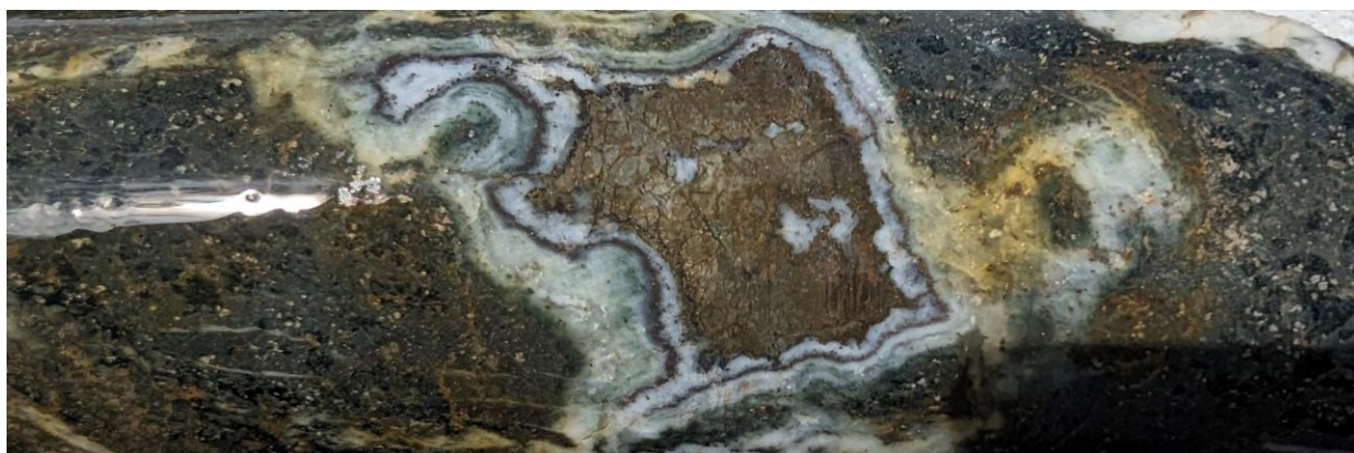
Diagram 6 : Banded, colloform gold bearing veins with internal zone of semi-massive pyrrhotite
