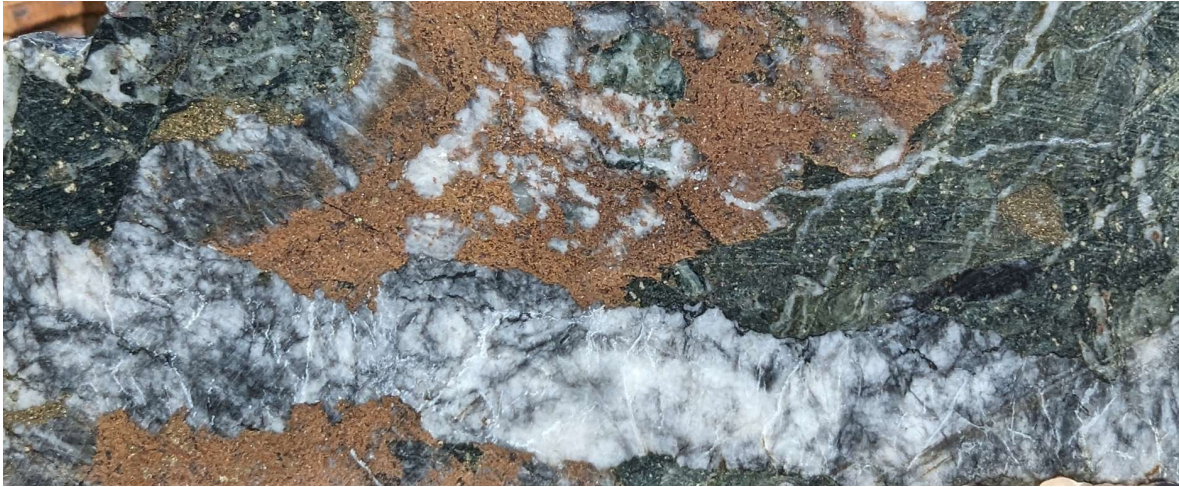
Diagram 7: Selective replacements of semi-massive sphalerite around gold-bearing quartz veins. SBC zone
