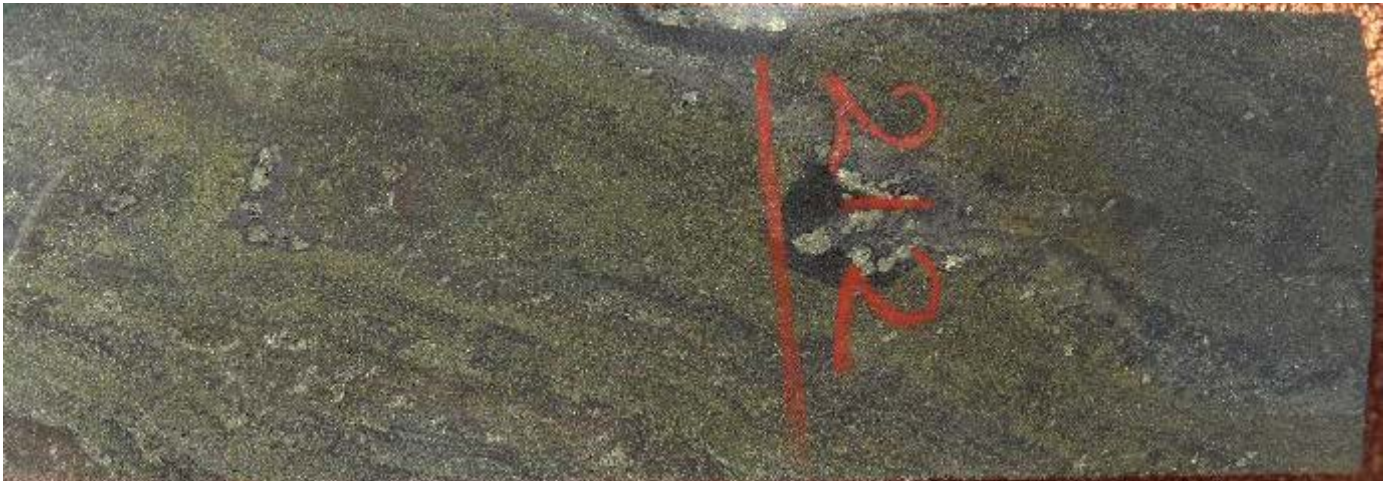
Figure 4 Drillcore from 212m depth from MMG – Havilah joint venture 2014 diamond drillhole BRK14DDO01A skarn mineralisation comprising laminated chalcopyrite (copper sulphide-brassy yellow colour) and dark grey magnetite (iron oxide) replacement bands. This interval carries more than 2% copper.
