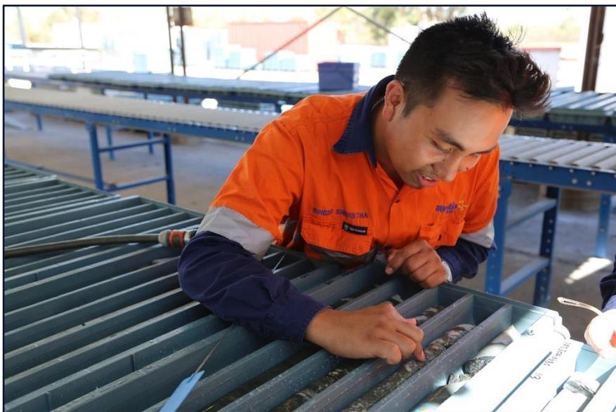
Figure 5. Exploration Geologist, Dinesh Shrestha, from the Cobar District exploration team in the Peak Mine core shed highlighting semi-massive sulphides in UD23CH0081.
