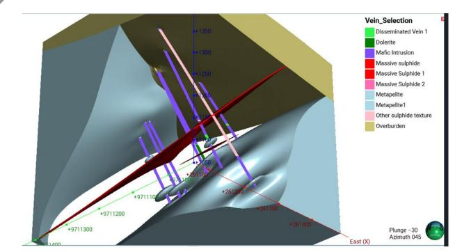
Figure 3: Leapfrog model of massive sulphide vein
