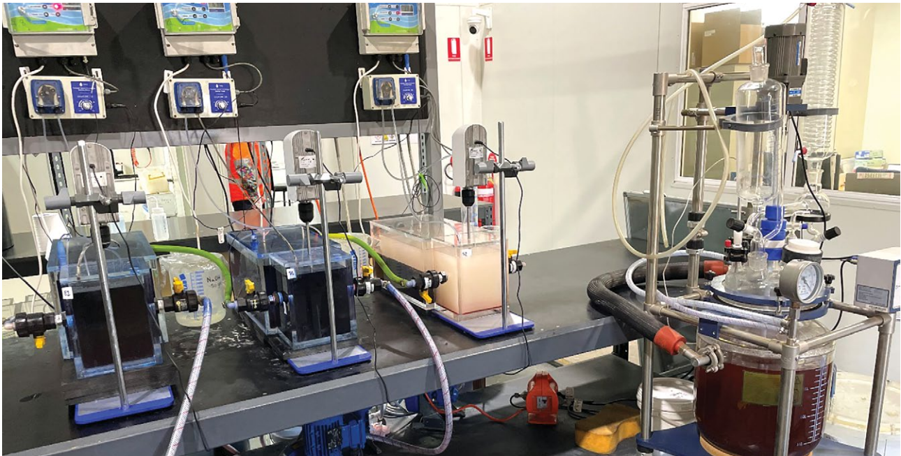
Figure 5 – Cobalt solvent extraction strip cell
