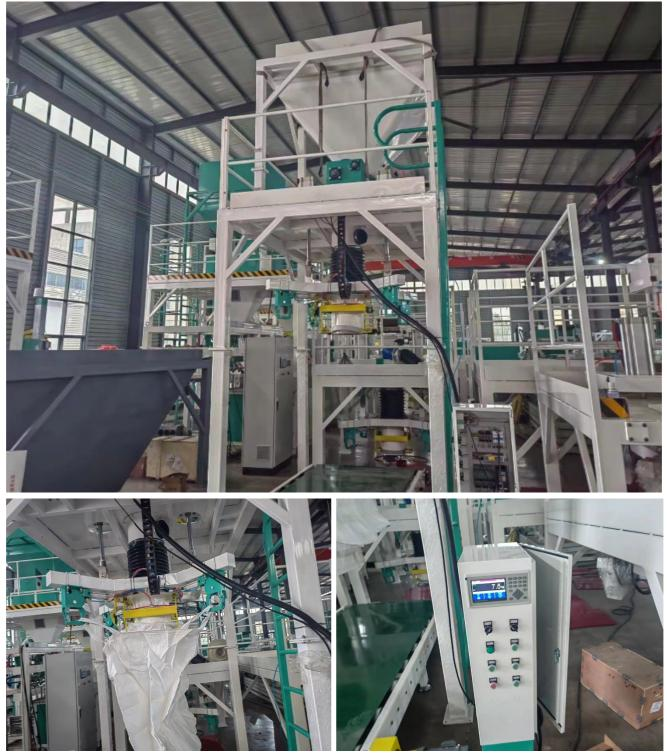
Figure: MgO Bagging Plant Shipped
