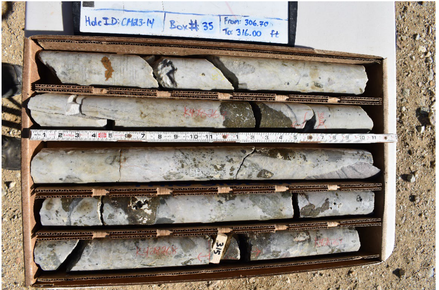
Figure 4 – Drill hole CM23-14, core from 306.7-316.0 feet, showing zones of sulphides.
