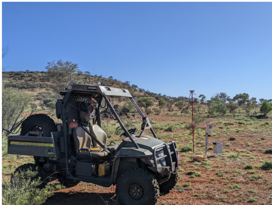
Figure 4: Image showing the gravity survey Base Station set up that includes a highly accurate GPS (on red pole) and gravimeter (silver box on ground). These are used for location reference and instrument calibration during surveys.
