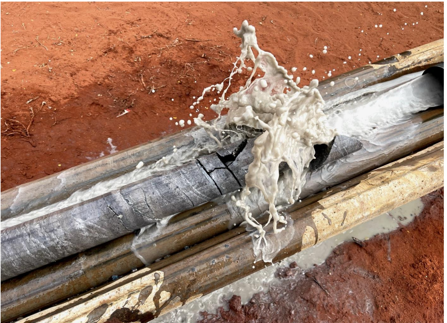
Figure 4: Diamond core being pumped out of the drilling rods at Aurora Tank (2023 re-drill)
