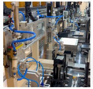
This image shows the robotic systems inside the automated lithium metal anode cutter. Here each anode is cut and formed before a vision system performs a thorough quality inspection and the anode is then passed to the cell stacking system.
