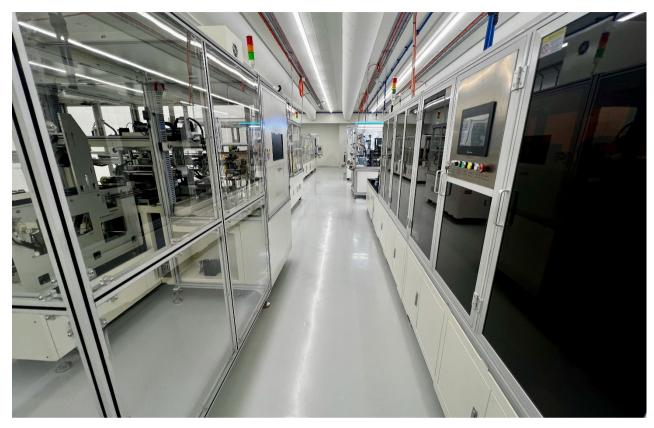
As lithium metal reacts with water, the cell fabrication itself is performed inside a dry room which eliminates almost all moisture from the atmosphere. In the image foreground are the automated anode cutter and pouch cell stacking systems, used to precisely cut the delicate lithium foils into anodes, then stack the anode, cathode and separator into a multi-layer battery cell.
