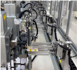
This image shows the automated battery tab welder. After the cell is stacked, the electrode tabs are each welded together to form the positive and negative electrodes for the cell. This complex process is performed completely automatically with robotic arms moving the cells through each of the 9 separate welding steps.
