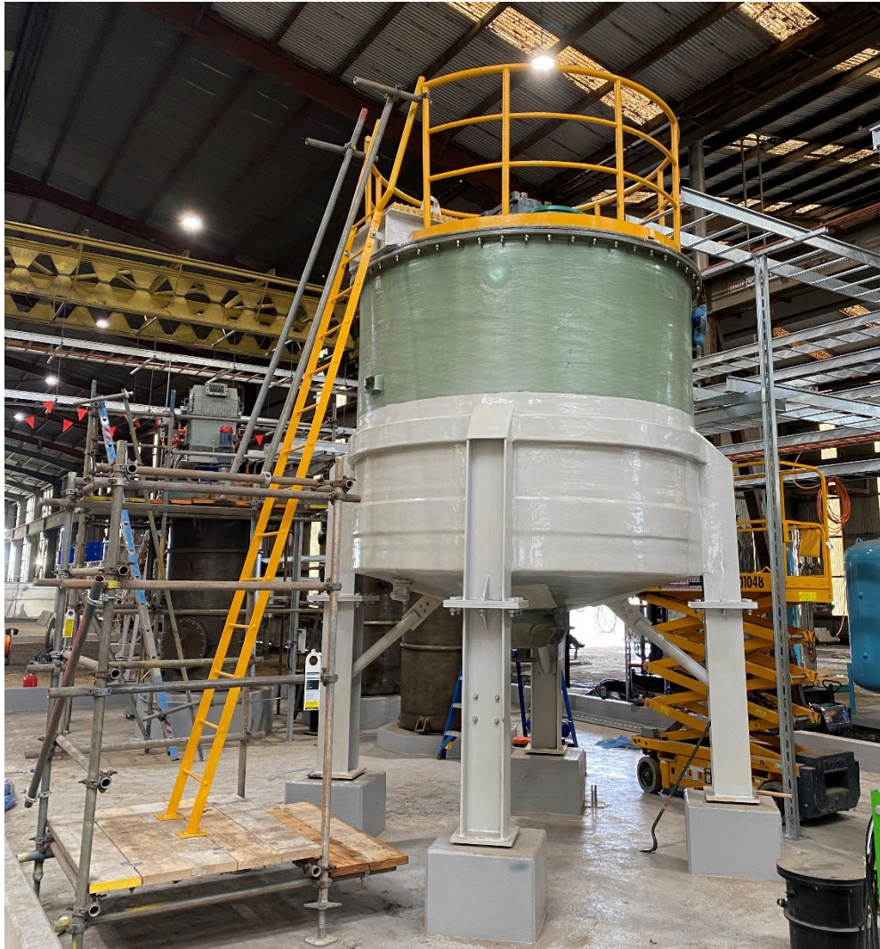
Figure: Thickeners with internal rakes installed (top) and carbon steel spoils welded ready for install (bottom)
