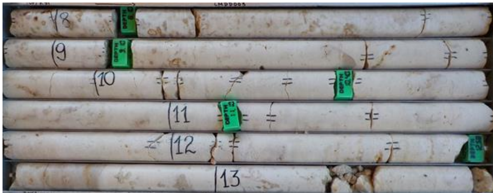
Fig 1 - HIGH purity Limestone (97% CaCO 3 ) from only 8m depth
