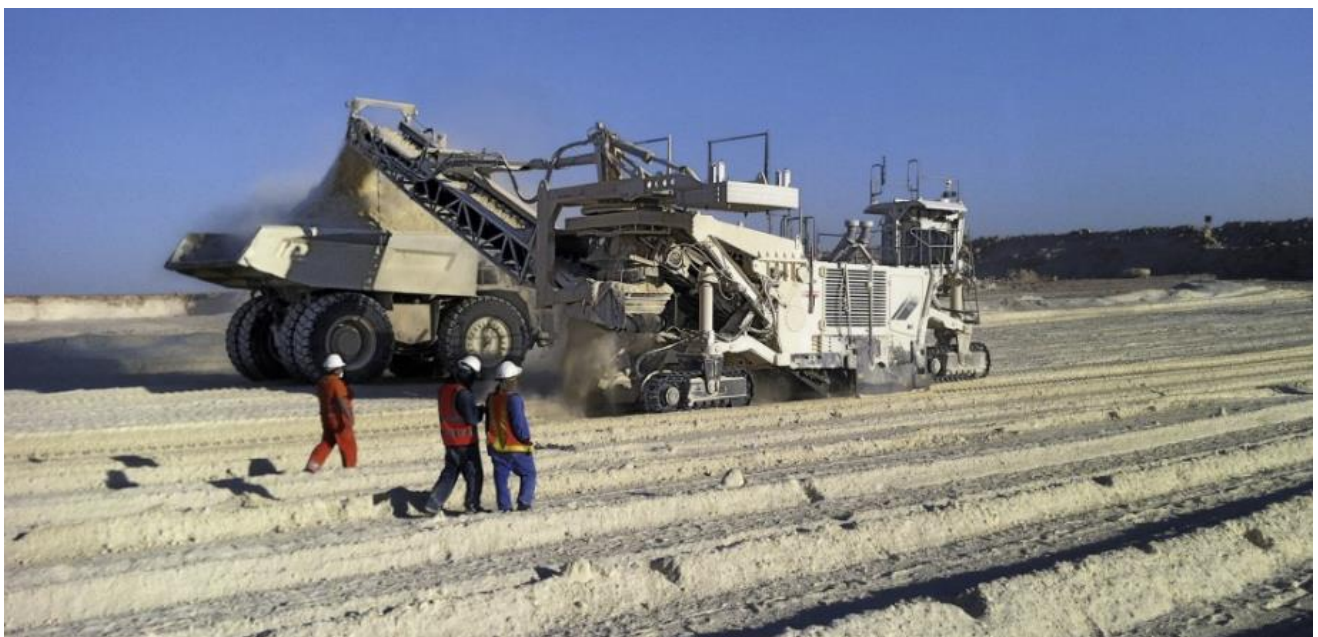
Fig 2 - Selective Miner – simultaneous Cutting, Crushing and Direct Loading of Limestone
