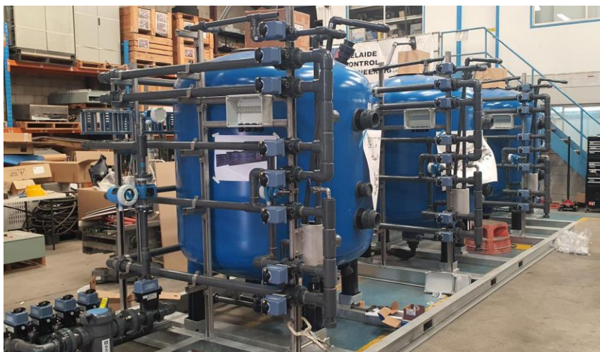
Figure 5: Progress of ion exchange module fabrication
