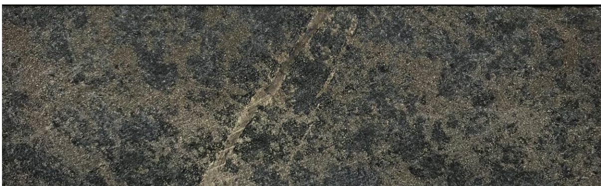
Figure 4.10: BNDDD006 – 81.00m. Komatiite dunite with leopard textured semi-massive interstitial sulphide & downward penetrating sulphide veins. Right of view is down the hole. Field of view from top to bottom ~47mm. (source: Hornsey, 2023).
