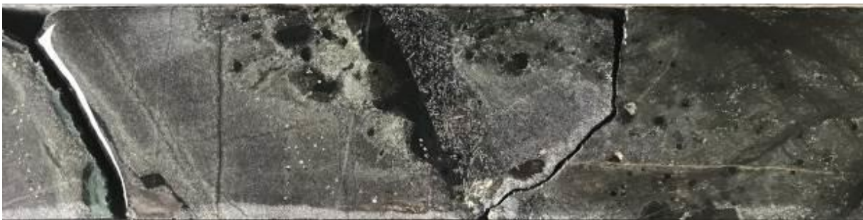
Figure 4.5: BNDDD008 – 48m - example of a chilled komatiite margin at the contact of two flow units. Patchy disseminated mineralisation noted in both flow units. Field of view from top to bottom ~45mm. (source: Hornsey, 2023).
