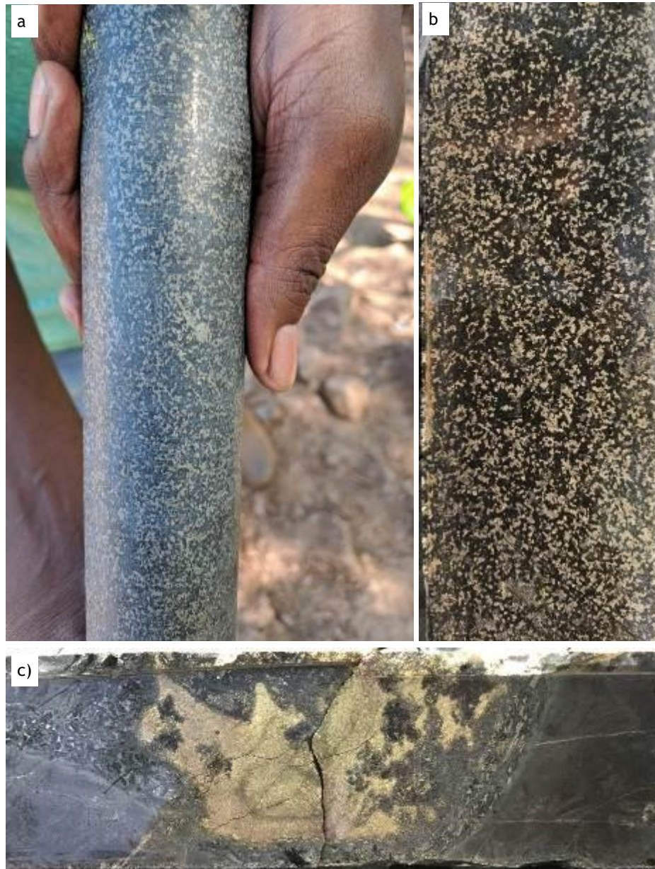
Figure 1: Core photographs of typical mineralisation at the Bend Nickel Deposit. a) and b) BNDDD002 – 379.38m – adcumulate dunite komatiite with net-textured magmatic sulphides from within a zone where the sample returned 10.33% Ni, 2.24% Cu, 0.10% Co and 4.30g/t Pt, 11.97g/t Pd, and 0.47g/t Au over 0.76m which relate to previous Company announcements (refer to Tables 2 and 3). Left (a) core sample, right (b) – cut core sample, NQ core. c) BNDDD005 – 99.90m - komatiitic basalt pillow lava intruded by massive sulphide with primary pyrrhotite-pentlandite-chalcopyrite showing dynamic process of absorption and generation of xenomelts at the massive sulphide margin (source: Hornsey, 2023). The sample returned 0.59% Ni, 2.47% Cu, 0.01% Co over 0.76m (refer to Table 2). NQ core.
