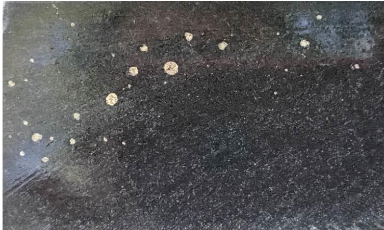
Figure 4.1: BNDDD008 – 43m – typical fine-to medium grained equigranular textured olivine adcumulate with patchy blebby/globular sulphides with magnetite. Field of view from top to bottom ~45mm. Right of view is down the hole (source: Hornsey, 2023).
