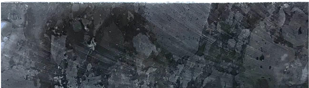
Figure 4.3: BNDDD001 – 72m – example of a dunite-komatiite, fragmented, blocky moderately magnetically susceptible, serpentinised, welded agglomerate. No obvious post-emplacement deformation. Field of view from top to bottom ~45mm. Right of view is down the hole (source: Hornsey, 2023).
