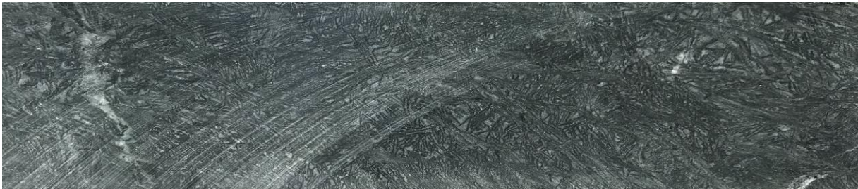
Figure 4.6: B1DD001 – 364.00m – pyroxene spinifex (medium grained). Random orientations. NQ core. Right of view is down the hole. Field of view from top to bottom ~45mm (source: Hornsey, 2023).
