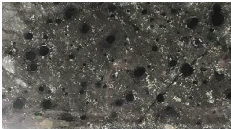
Figure 4.2: BNDDD008 – 43m – example of a vesicular dunite komatiite with chlorite (?) infilled vesicles and patchy carbonate alteration. Provides evidence for extrusive nature of the Bend Nickel Deposit flow units. Field of view from top to bottom ~45mm. Right of view is down the hole (source: Hornsey, 2023).
