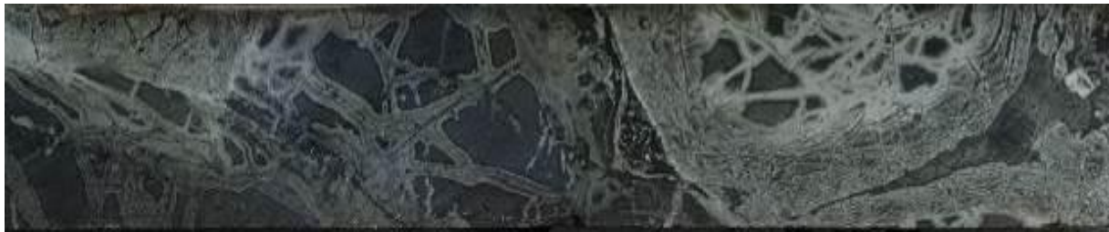
Figure 4.4: BNDDD001 - 271m – example of a fine-grained komatiitic basalt with pervasive chlorite alteration. Rounded structures with intensely altered and fractured margins and wider-spaced interval fractures and alteration. Interpreted as pillow lavas (flow-tops). Right of view is down the hole. Field of view from top to bottom ~45mm (source: Hornsey, 2023).
