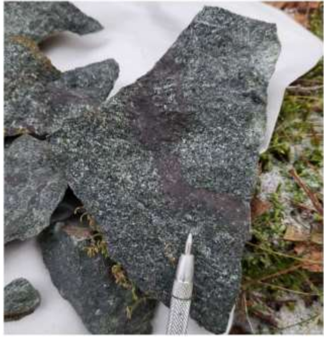
Figure 3: Dark REE vein in green actinolite-tremolite skarn in the project area.
