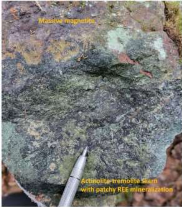
Figure 2: Patchy REE mineralisation in actinolite-tremolite skarn in the project area.
