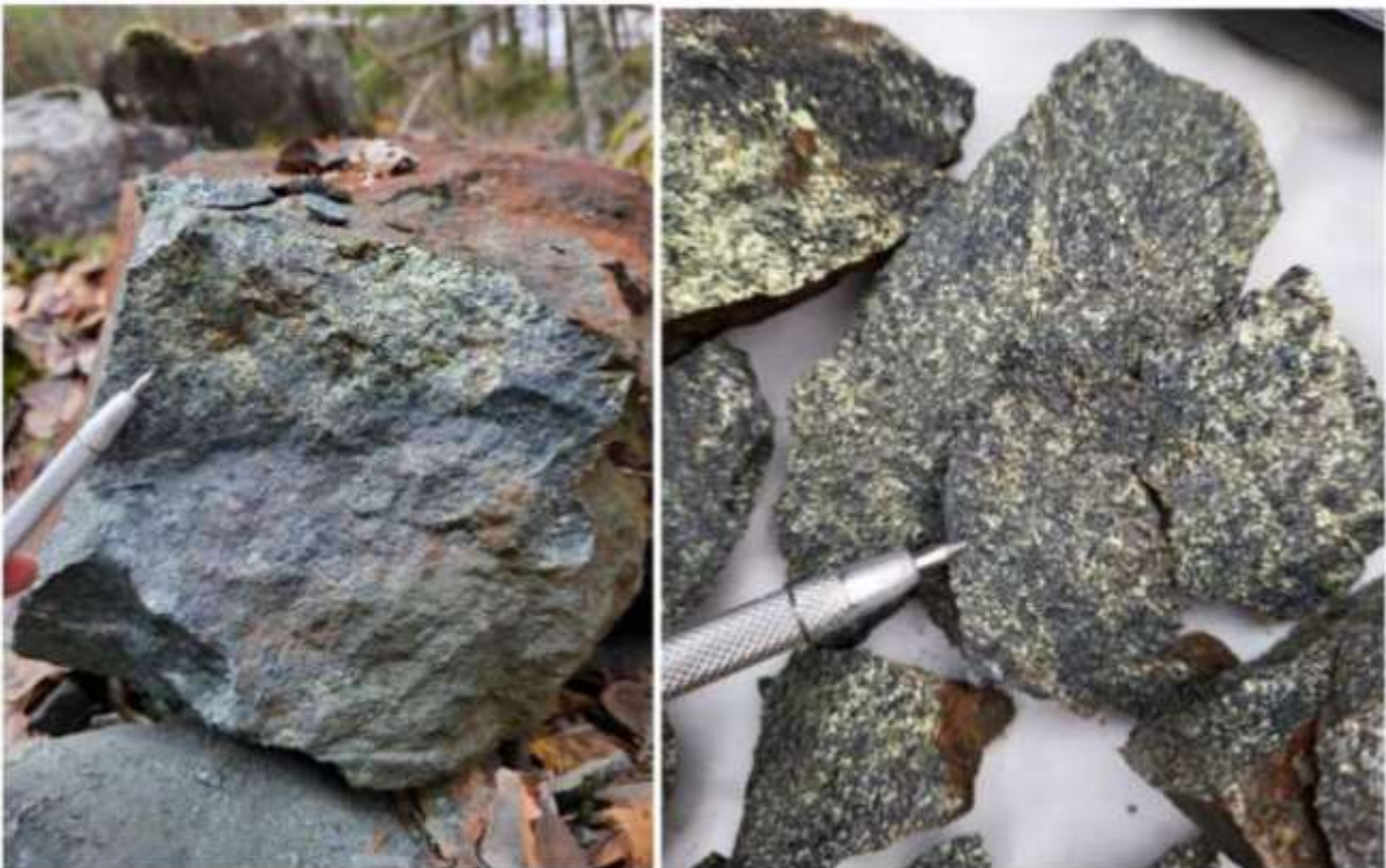
Figure 4: Lenses and clusters of chalcopyrite in massive magnetite boulders (GYTR015).
