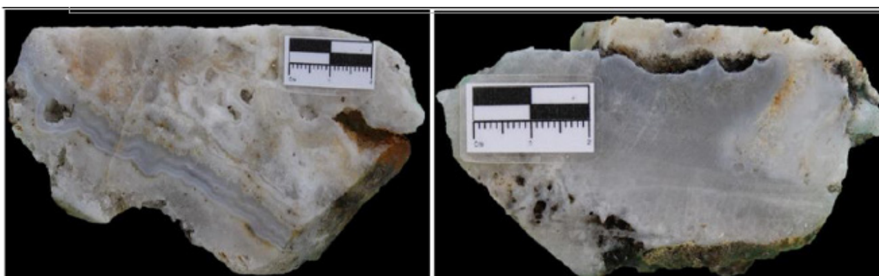
Figure 4: Left: Drill core from RRD027 (79.6m) showing vuggy, crystalline quartz crosscut by finely banded opaline quartz veins. Interval assayed 15.93 g/t Au, 108 g/t Ag (17.23 g/t AuEq) from 79.3-79.7m. Right: Drill core from RRD028 (103.6m) showing predominate massive chalcedonic quartz. Interval assayed 7.44 g/t Au, 40.6 g/t Ag (7.93 g/t AuEq) from 103.2-105.4m.
