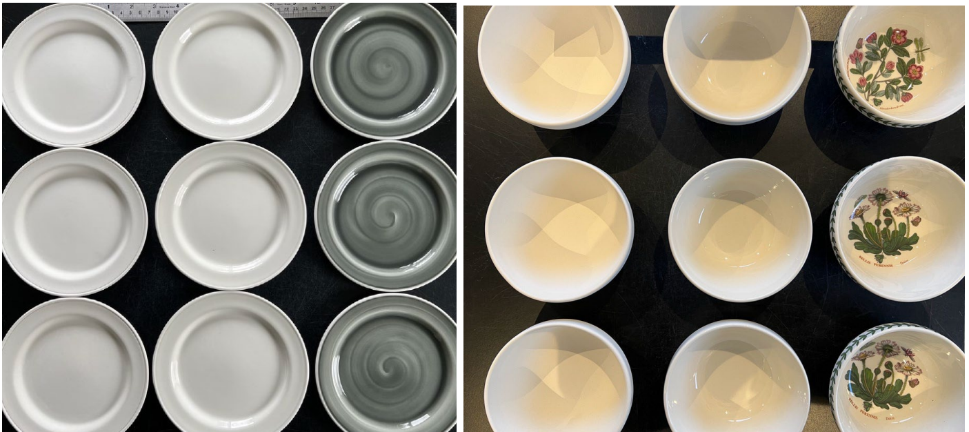
Figure 2: Trial-fired ceramic plates and bowls, manufactured in biscuit (unglazed), glazed and decorated forms (left to right), comprising of trial standard, O/F sample and U/F sample (top to bottom). The trials, which deemed that no visual differences were detected between the trial standard and sample plates, successfully produced industry-accepted standard of ware across all aspects.
