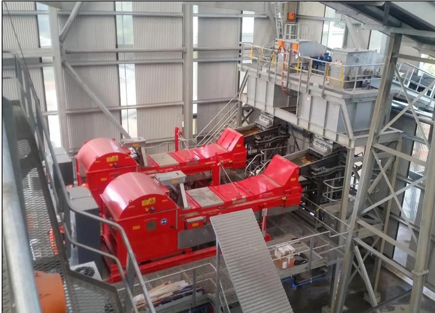
TOMRA Ore Sorters in operation at the Renison Tin Mine, Tas.
