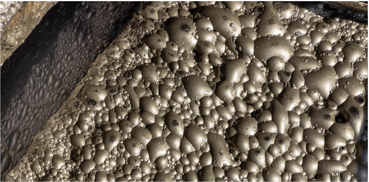
Figure 2 Copper concentrate production through the flotation circuit
