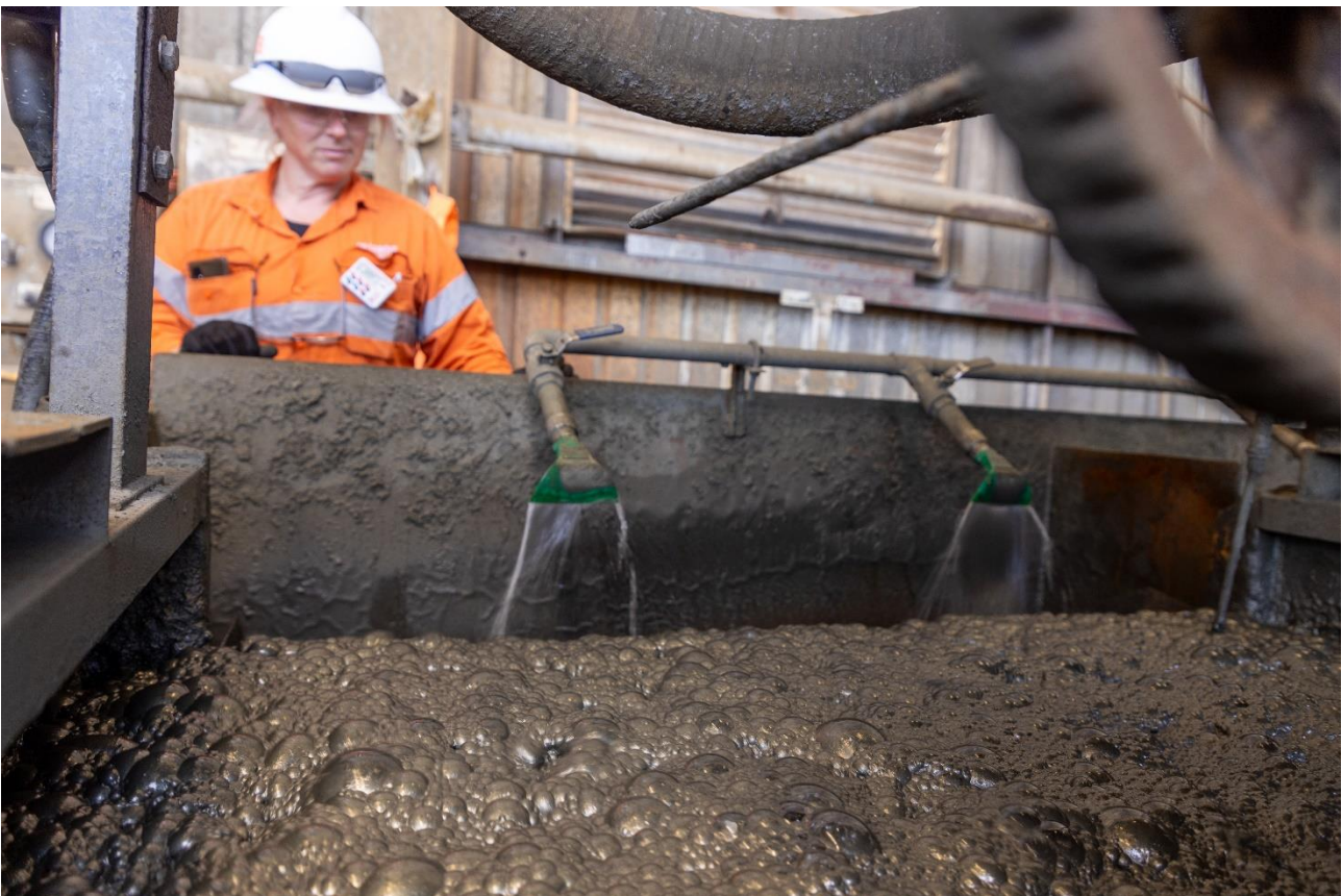
Figure 2 Copper concentrate production through the flotation circuit
