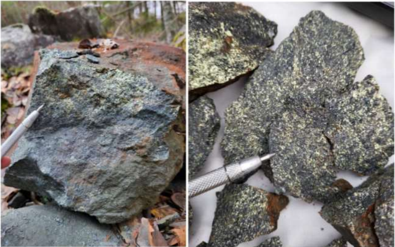
Figure 6: Lenses and clusters of chalcopyrite in massive magnetite boulders (sample GYTR015, which reported > 2.5% copper, and 184 ppm total REE + Y, see Table 1 below, for analyses from ALS laboratories). The chalcopyrite is present as disseminations and fracture coatings and is the only copper mineral observed. There is approximately 10-20 % chalcopyrite in the sample submitted for analysis, which is being re-analysed with a higher upper analytical limit to determine the total concentration of copper. The results from this re-analysis are expected within approximately 4 weeks. 493933 East/6597081 North SWEREF99.
