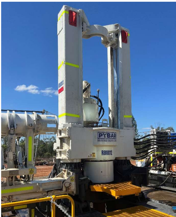
Figure 1: Pybar raisebore rig in place reaming
