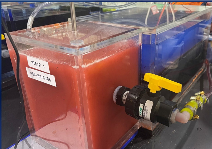
Cobalt Solvent Extraction Strip Cell
