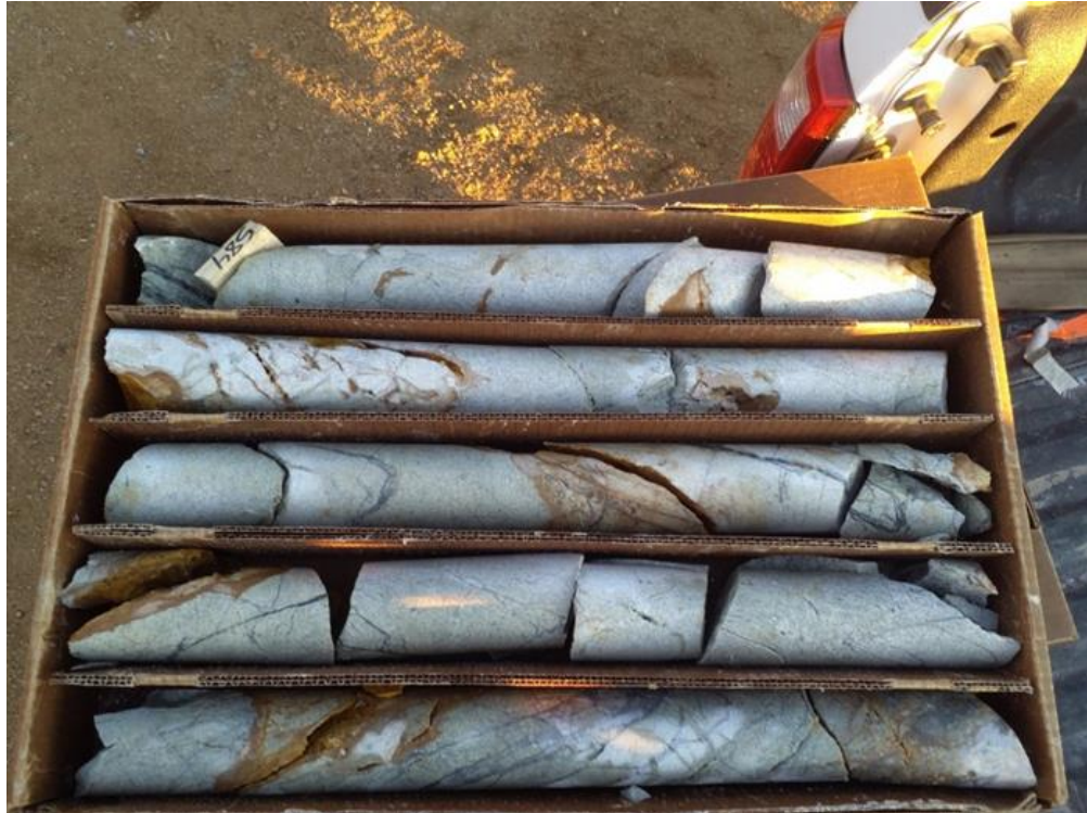
Core from GDD02 from 178 m to 181m downhole which assays 40 g/t Gallium Stockwork and sheeted quartz-sulphide veins. Quartz-sericite-pyrite alteration
