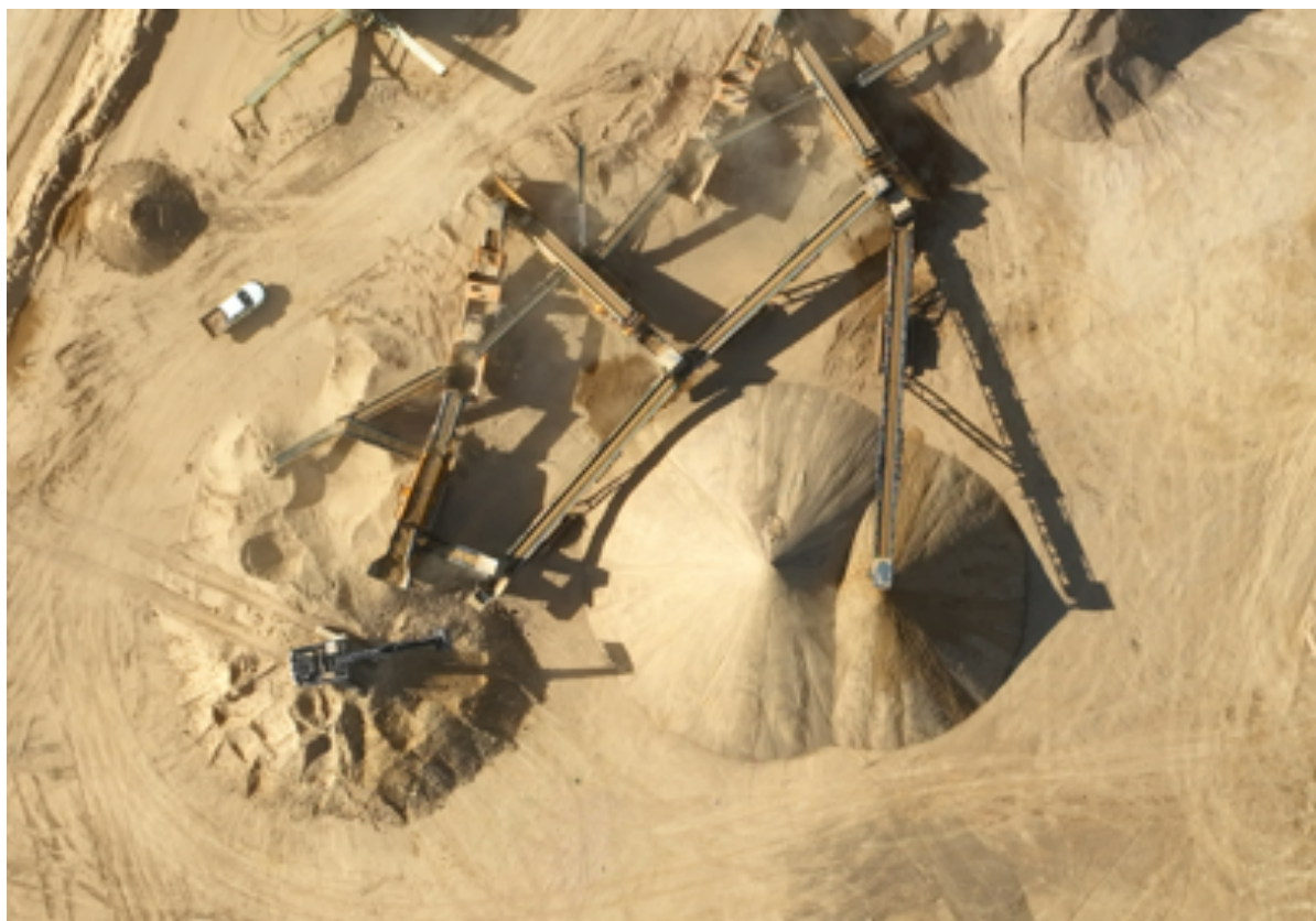
Figure 5: Crushing plant overview.
