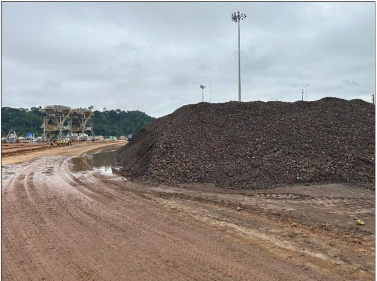
Figure 20: Manganese ore stockpiles waiting to be loaded onto ships at the port of San Pedro, Côte d'Ivoire – recent photo by Mako Director
