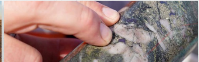
Quartz vein (15cm) with bornite (blue), pyrite and minor chalcocopyrite at 221.2m
