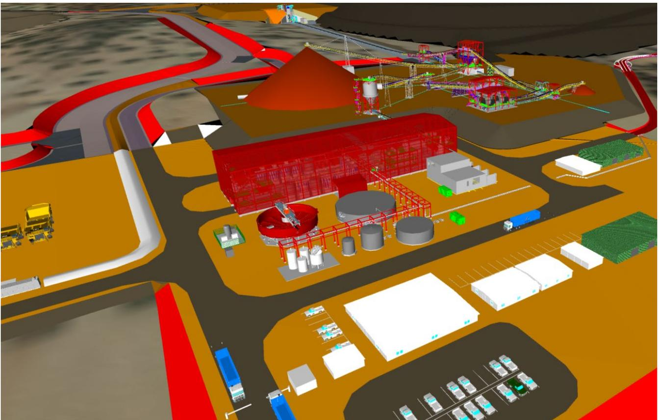
**Figure 4.** Oropesa Project 3D Model Infrastructure - Mineral Process Plant, Offices, Mine Contractor Area, Crushing and Ore Sorting
