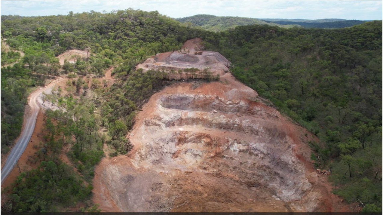
Sherwood West Pit 1 – mining the up dip extension of structure outcropping at top of hill
