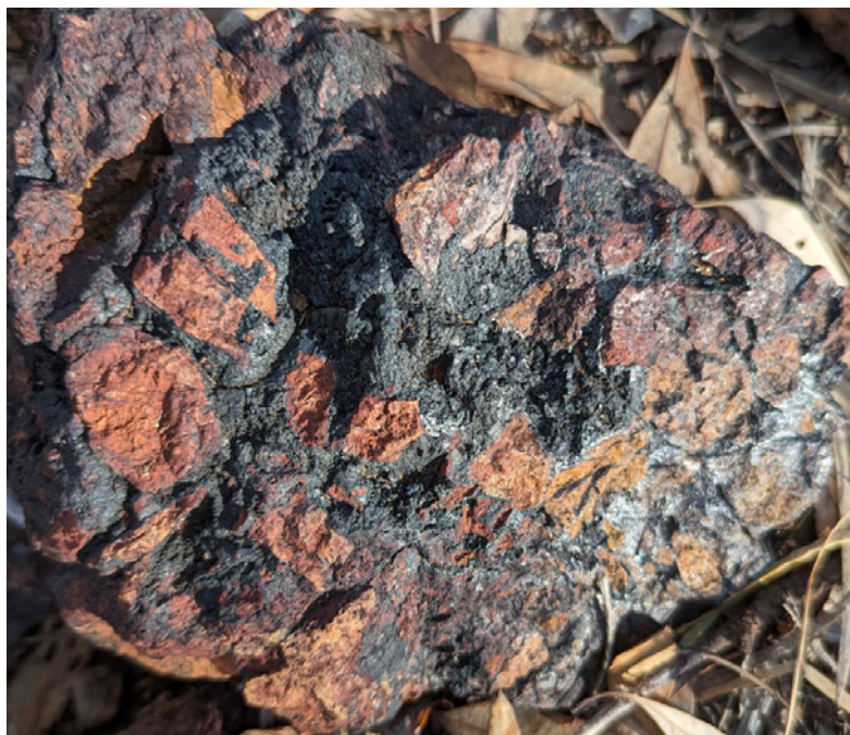
Figure 5*. Example of Fe-Mn gossanous breccias outcropping at the Alpha Gossan, Camp Gossans, Mt Oxide Project
