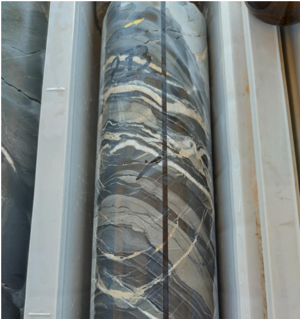
Figure 1: Diamond Core from Carpark hole PCP008. Stockwork quartz veining with ankerite within anomalous zinc zone.
