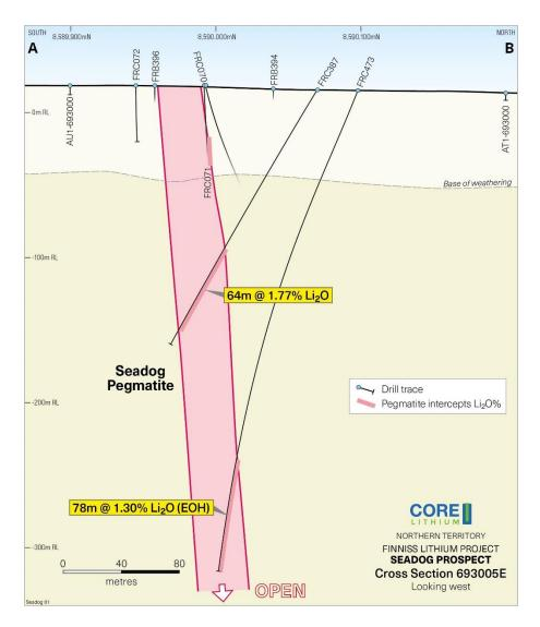
Figure 3: Seadog Cross Section
