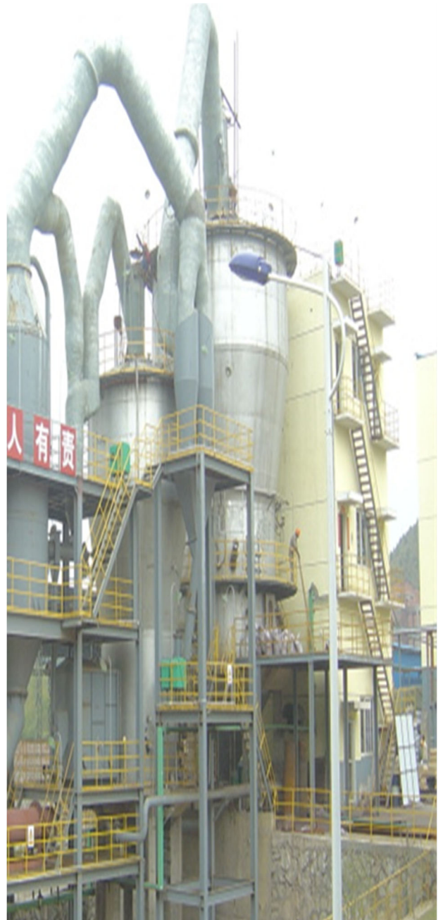
BGRIMM 200tpd Two-Stage Fluidized-Bed Roaster
