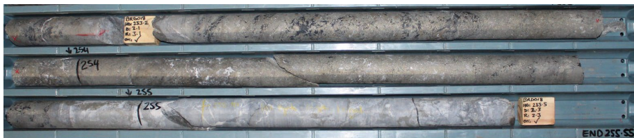
BRD018 , massive sulphide mineralisation (253.0-255.5m)
