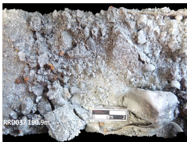
Figure 4: Photos of core specimens from the Susi vein drill hole RRD037(left) and the Pertama vein drillhole RRD039 (right). RRD037-190.9m is a milled and cemented fault breccia with rounded fragments of quartz and argillic altered volcanic. Part of a 1m wide sample interval that assayed 8.09g/t Au, 17.8g/t Ag (8.3g/t AuEq) from 190-191m. RRD039-187.6 is crystalline quartz with faint, fine bands of glassy quartz. Part of a 0.7m wide sample interval that assayed 2.75g/t Au, 55g/t Ag (3.41g/t AuEq) from 187-187.7m.
