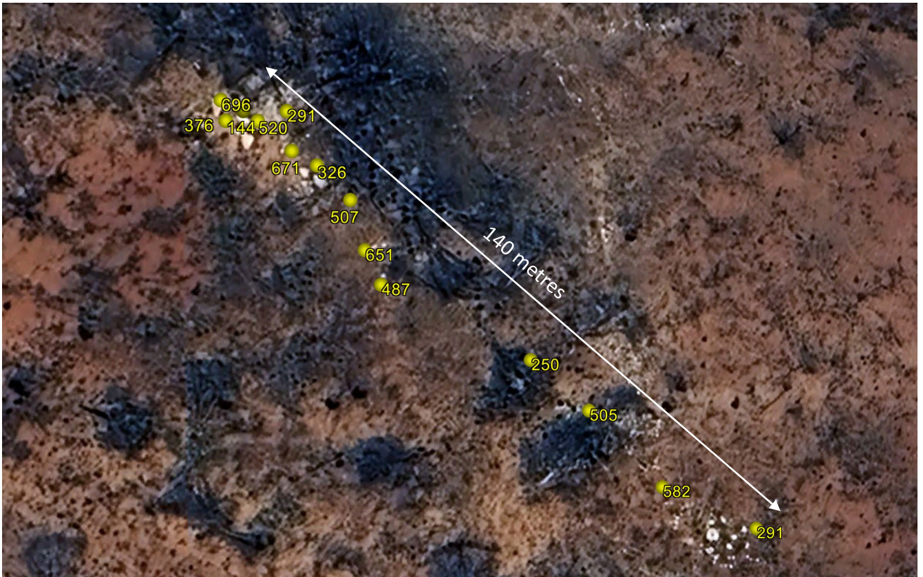
Figure 3. Image of outcropping pegmatite (white) with rock chip locations and Li 2 O assays results (yellow).
