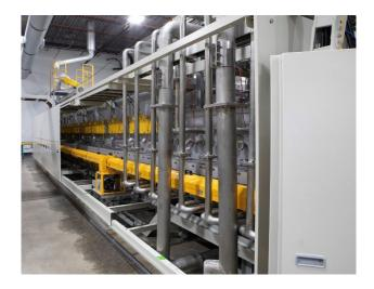
NOVONIX 13.5 m long pilot roller hearth kiln (RHK) with partial insulating panels removed displaying assortment of gas handling plumbing, banks of resistance heaters (yellow rectangles, top), and roller conveyance mechanism (yellow, middle).
