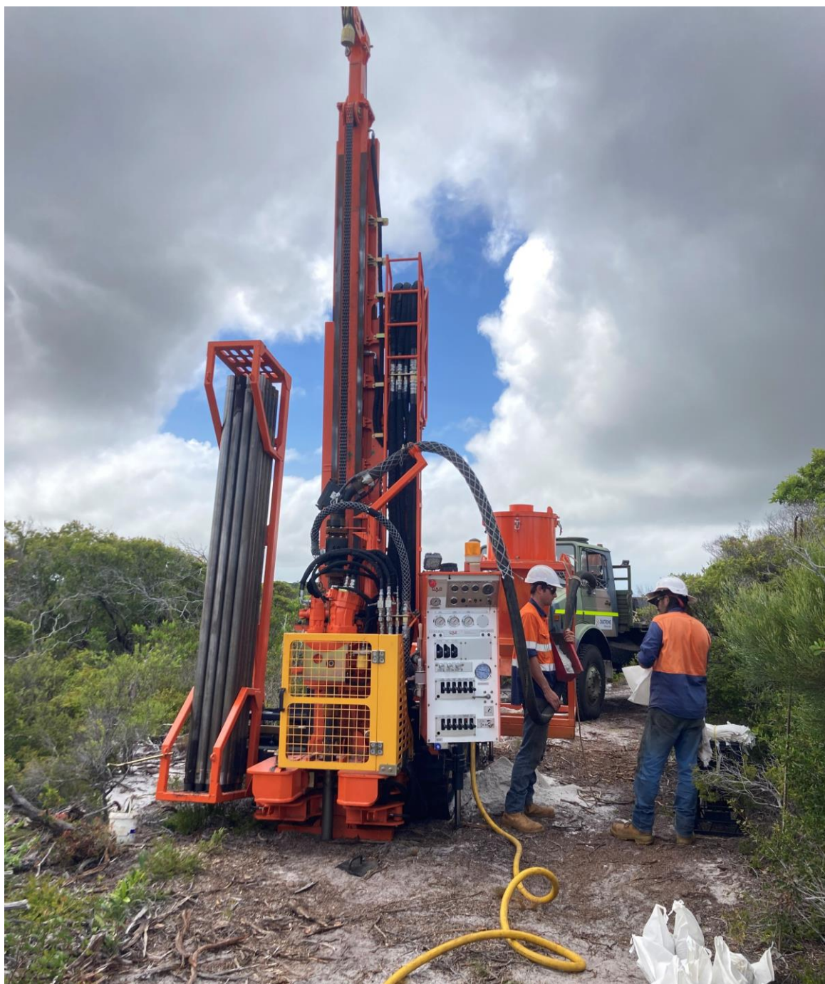
Figure 4: Diatreme Resources' Aircore drill rig showing sub-sample collection after the riffle splitter.
