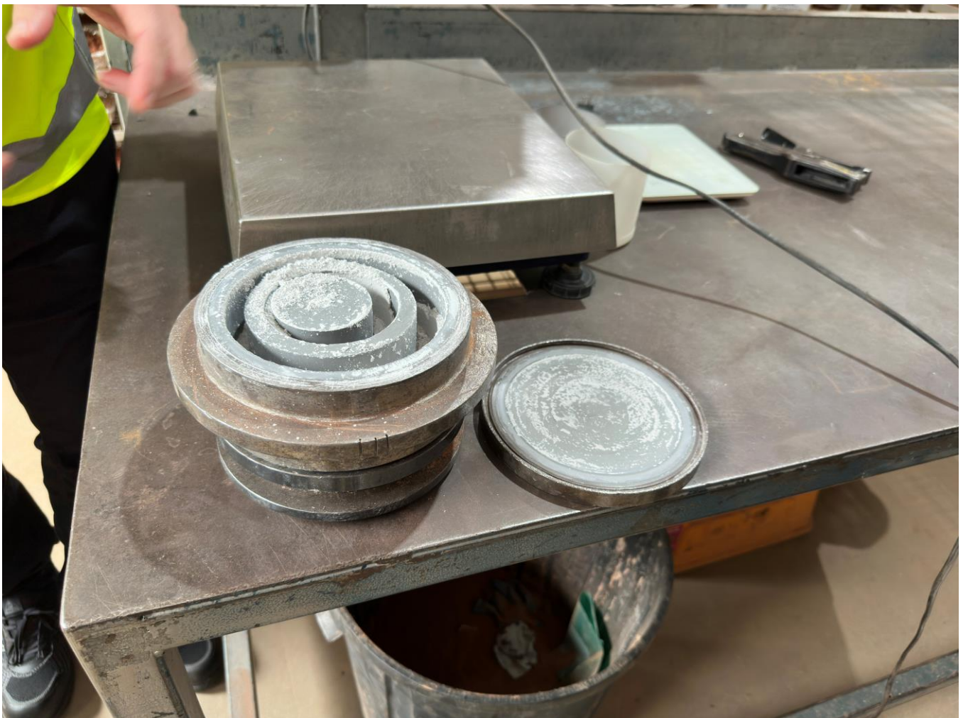
Figure 5: Tungsten carbide pulverising bowl used to ensure Fe-Cr contamination is minimised during sample preparation.
