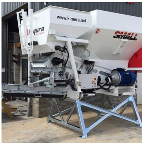
Figure 21: Small mobile concrete batch plant
