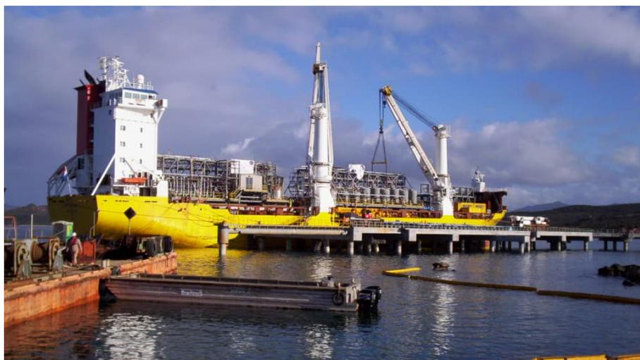
*Figure 30: HLS transporting prefabricated modules*
